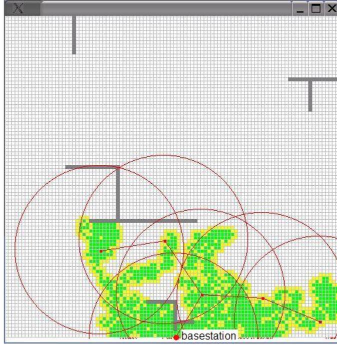
**Fig. 3.** A screen-shot from a typical simulated run of the basic communicative exploration algorithm where the robots constantly keep in contact with an immobile base-station. For this purpose, an utility function penalizes the motion that lead to a loss of a link in the ad-hoc network formed by the robots. Though being important for some application scenarios, this approach limits the maximum operation area of the robots.
