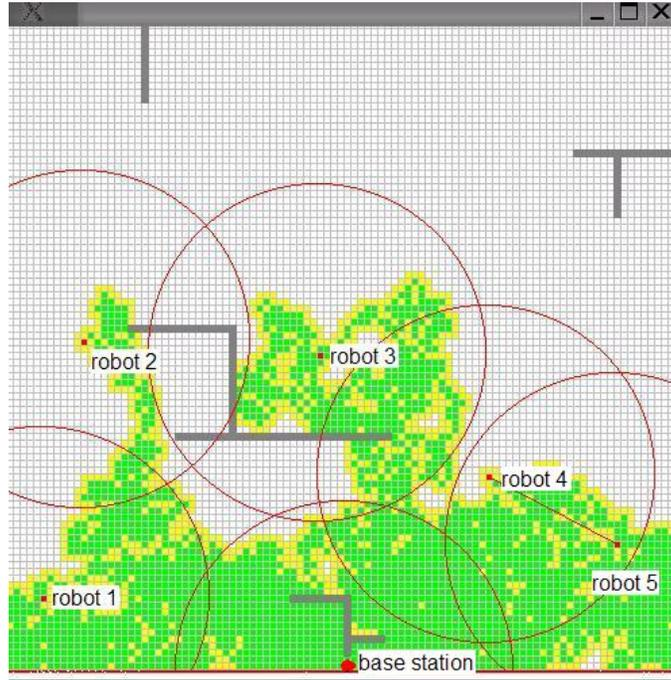
**Fig. 1.** *The frontier-based exploration algorithm does not put any constraints on the spread of the robot pack. The robots soon drift far apart and communication is easily lost. In the above screenshot from a typical simulated run, only robots 4 and 5 are in each others cell and hence capable of communicating with each other.*
