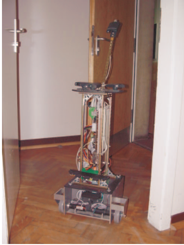
Fig. 5. The inside core of the RoboGuard base, a commercial semi-autonomous robot for surveillance applications.
