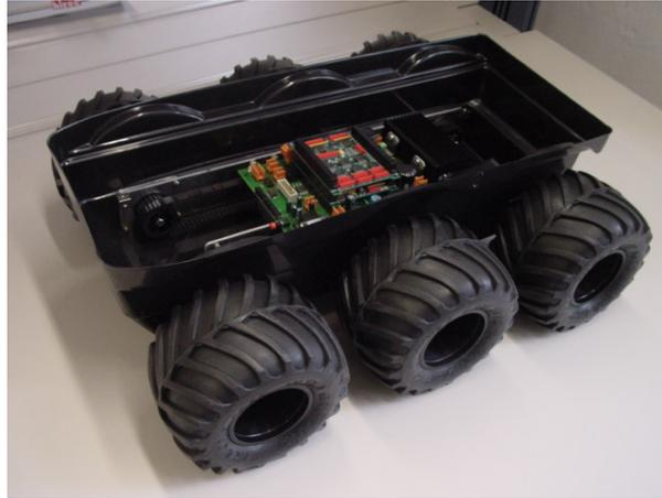
**Fig. 7.** The new mobile base with six actively driven wheels.
